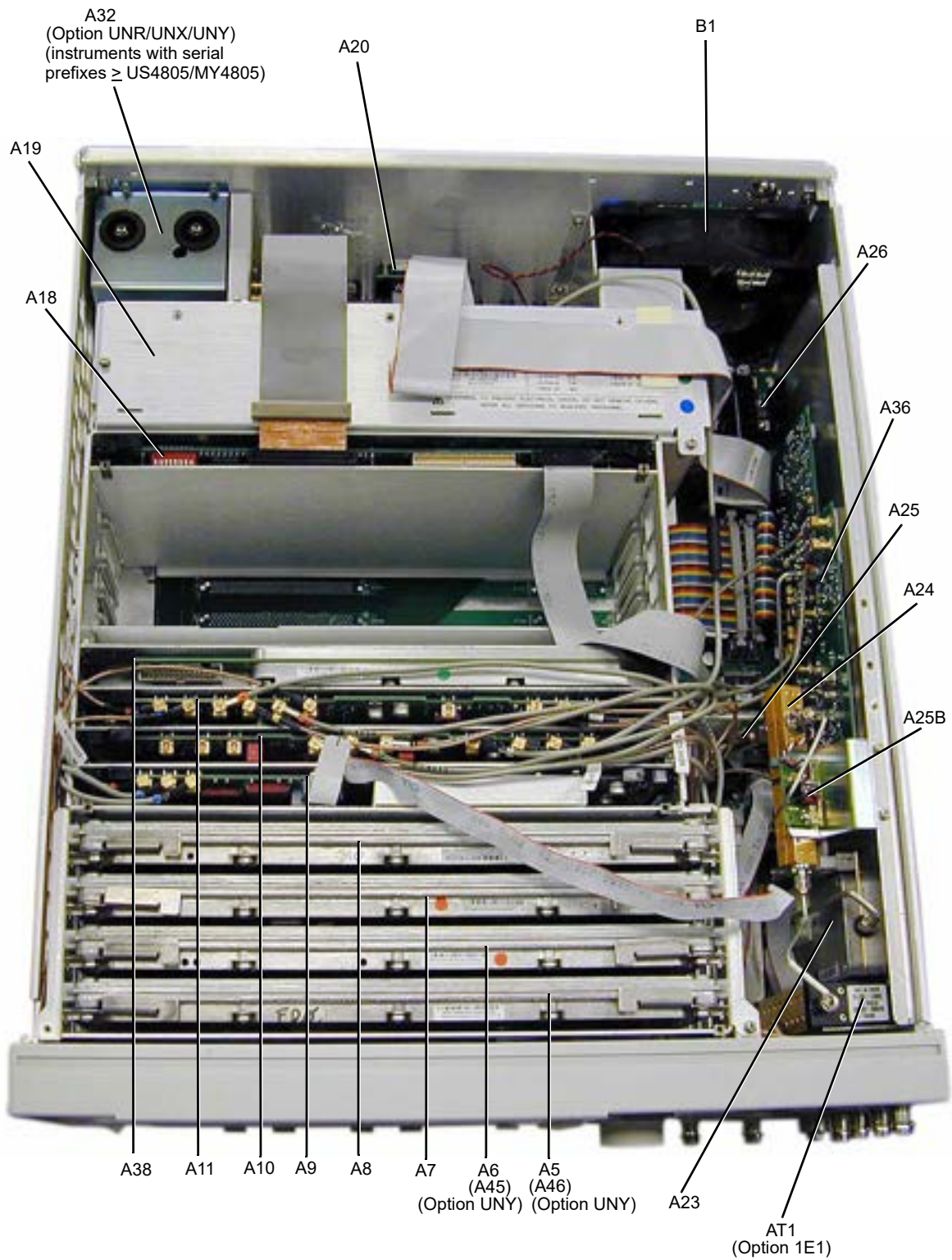
Figure 2-5 Assemblies from a Top View (E8257D Option 550/567)
