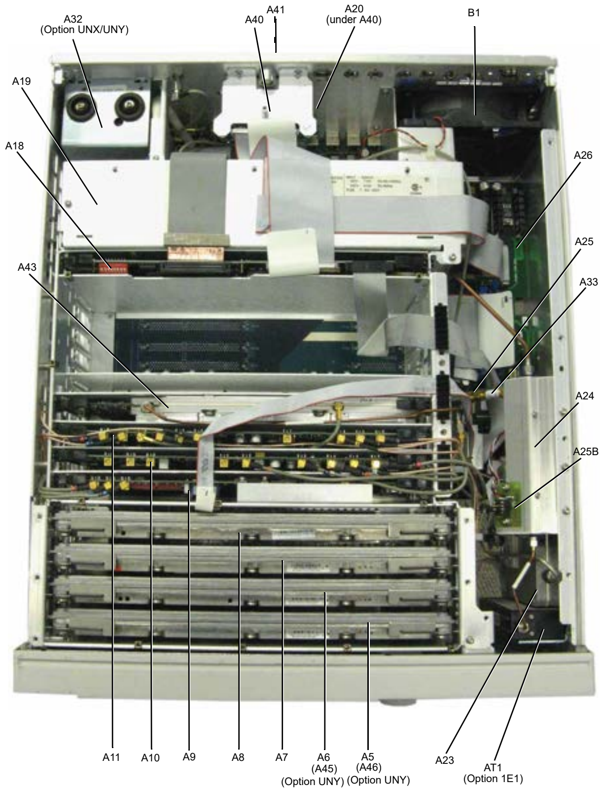
Figure 2-4 Assemblies from a Top View (E8257D Option 521)
