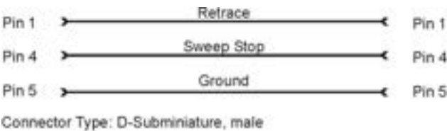
Figure 2-9 RS-232 Pin Configuration
