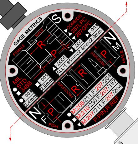
INTERFACE GEOMETRY FOR 1.85mm, 2.4mm, 2.92mm, 3.5mm AND TYPE N IS PROVIDED FOR BOTH GENDERS WITH REFERENCE PLANE CRITERIA **CLEARLY MARKED**
