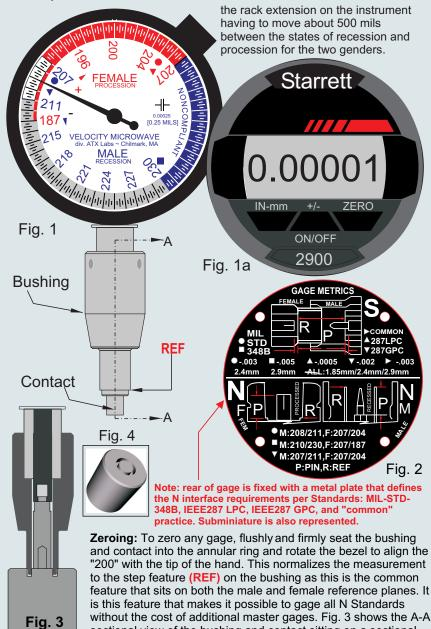
sectional view of the bushing and contact sitting on a sectional
