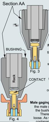
Fig. 5 Panel 2 subminiature SMA Gaging in general is not unlike checking tire tread depth, the technique is the same though it requires greater accuracy and precision: a fixed bushing rests on one plane or grade and a movable contact rests on a second plane. The dial records the differential grade. Velocity Microwave's gages are designed to be both user friendly and accurate, and the stainless parts are warranted against defect for a period of 10 years.
